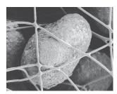
Gas contaminants must pass through tortuous pathways coming in intimate contact with the carbon. The fibers anchor themselves to the carbon using only 1% of the carbon's surface helping to maximize the contaminant's exposure.
